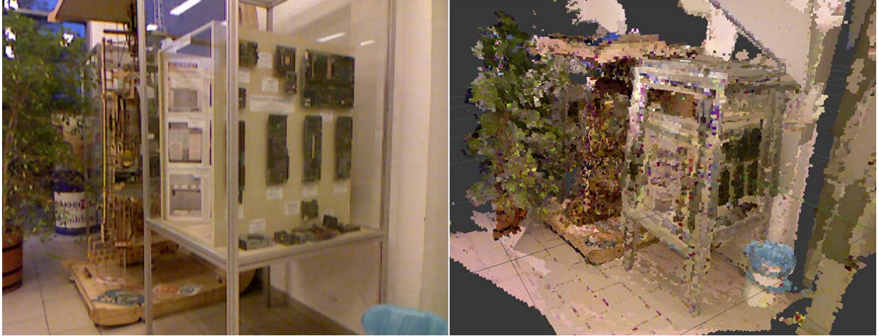
Figure 5. A voxel scene constructed from 30 nodes (right) using 1\text{cm}^3 voxels. RGB image from one of the nodes for comparison (left).
